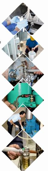
For samples (such as turbine and hydraulic systems), UCVD containers are the best option when cleanliness testing is important, the container should be fully clean, and no contamination should enter the sampling process. Due to internal vacuum pressure, there is no need to use a sampling pump.
